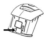
To dispose dust, press the lock button.
